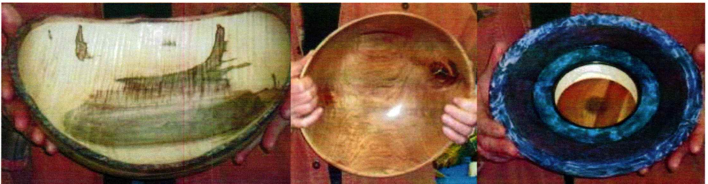
Kevin showed a large Ambrosia natural edge Maple bowl with a wax finish which he says he has not finished it yet, then a Hickory bowl with a smooth edge turned wet twice using a microwave to dry the wood in between sessions. He found warpage was kept to a minimum this way. He had sealed it with Anchor Seal in between which was drawn into the fibers during the microwave process. It was also waxed using Crystallon base wax, and finally showed a Maple (?) bowl which he turned and decorated with a chatter tool before applying dye as an experiment.
