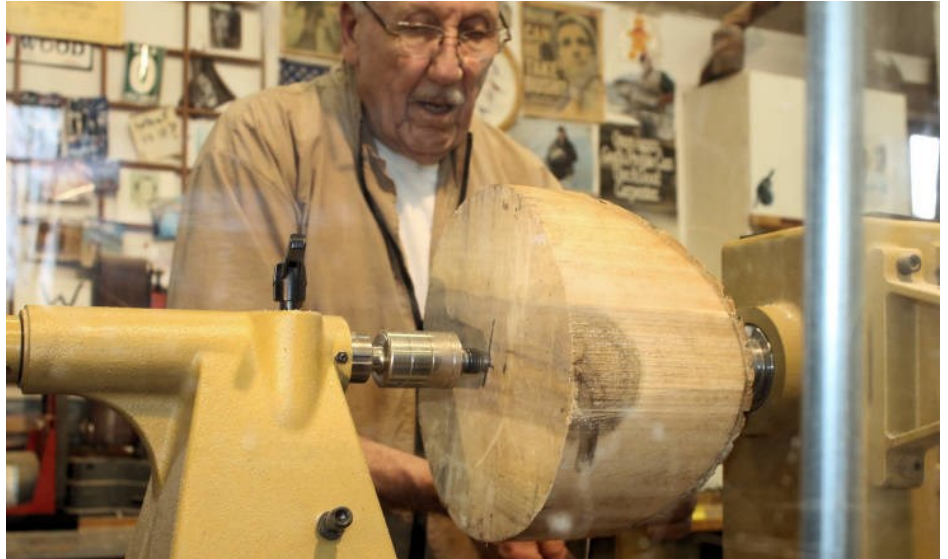
Steve mounts a blank on the lathe in preparation for turning a Natural Edge Bowl. He stressed that the high points line up evenly as well as the low points before you begin.
