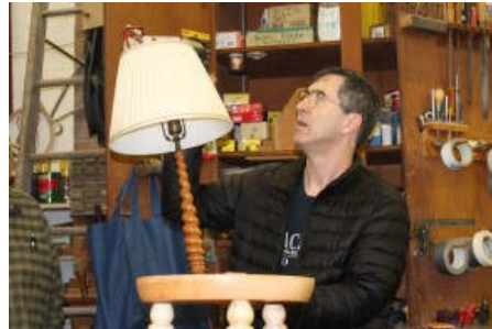
Mike's lamp with a graduated twist stem. He drilled through the middle for the wire.
