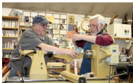
4. Lenny Mandeville helps Lenny Langevin mount the metal tang of the gouge into the new handle.
