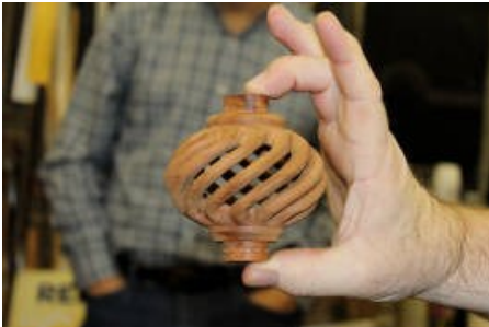
Mike Veno shows us a hollowed out oval sphere which he also removed part of the middle through indexing to create a spiral effect. Interesting concept and more work than one might think involved here.
