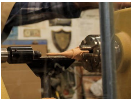
the finial has been shaped and is ready to be parted off.
