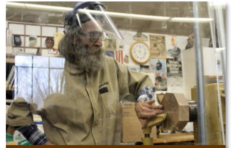
Ian has mounted his bowl blank on the lathe in preparation to turning the bottom.
