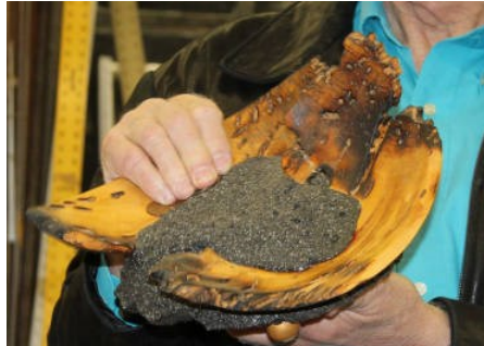
Ken's natural edge box elder bowl which blew up as it was being turned. He put the pieces back together with the help of some coffee grounds and glue, painted it black and
