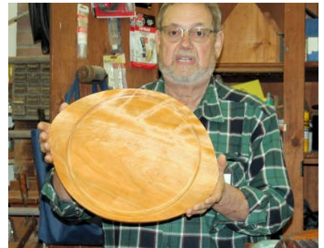
Joe showed us this large birch platter the wood for which came from Lenny Langevin. It was 25 years old from his basement. Joe turned the bottom then used a jig to join the top to get an adjustable French curve which he then cut out on the bandsaw before finish
