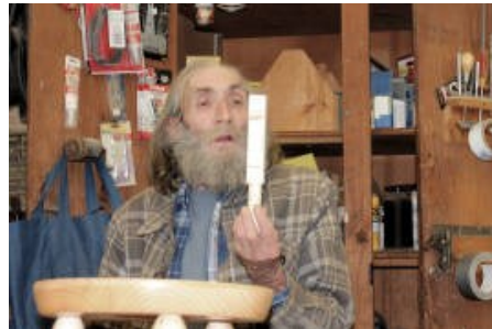
In response to questions of how he accomplished the hole spacing for the ring bowl, Ian showed us a simple jig, a drill post
