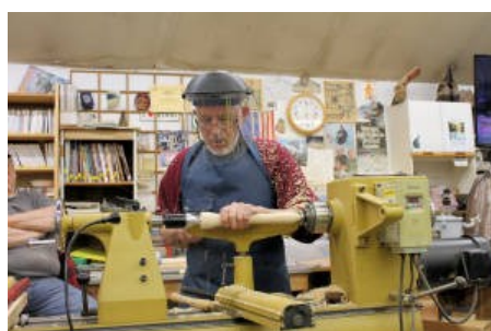
2. The handle has been turned around as Len gets ready to shape the front.
