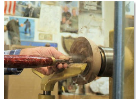
Ian proceeds to hollow out the inside leaving a base for the ring finial to sit on.
