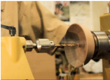
Ian drills a small hole for the ring finial to be seated on.
