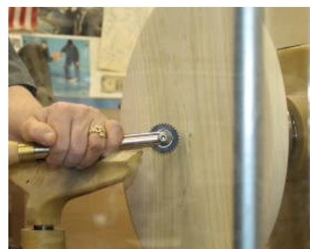
Kevin shows us the correct way to hold the Sorby Chatter Tool beginning in the center with the bevel making contact with the wood.
