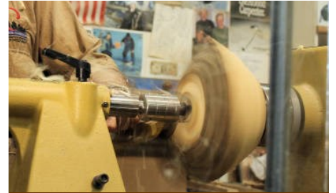
Bottom finished, tenon formed, Steve has
