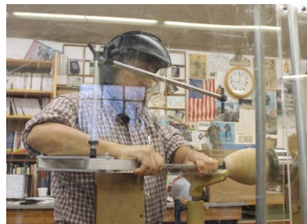
Pablo emphasizes that before you can pierce something, it must be turned thin Here he demonstrates this process on the lathe.
