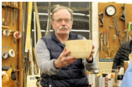
Billy Martin Shows us a small bowl with decorative lines added to the outside turned from birch. he used CA glue on the pith inside. He burned the rings on the outside and used OB's Shine juice (alcohol & shellac) as a finish and minwax.
