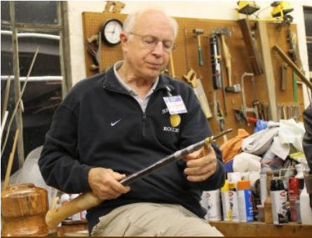
Allan holds one of his large handled turning tools made using threaded pipe. Diameters include 1/2", 3/8", 1/4".. He mentioned vibrations in using them. Ian offered that he would be better off using a solid bar to reduce vibrations. Threaded joints weaken the cutting end further.
