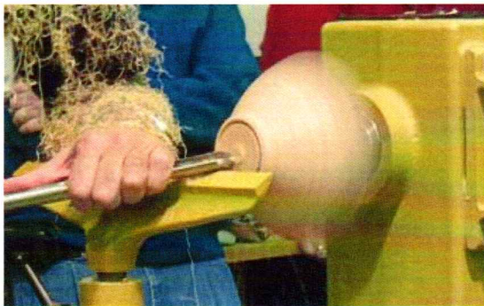
Preparing the tenon before remounting
