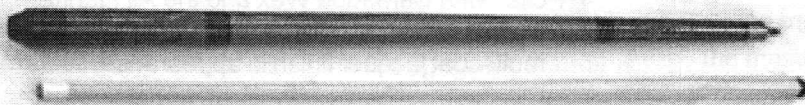
Jeff Keller's pool/billiards cue - maple, cherry burl and ebony with spar varnish finish - spent some time at Wally's shop lining up stock for boring hole accurately for proper alignment of both sections
