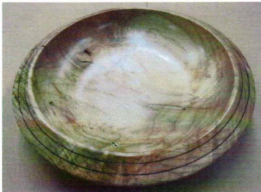
Ron Robertson displays a Maple bowl inspired by Jimmy Clewes. It has a brass inlay groove formed first into a v shape. Then brass powder and resin was mixed together and smeared over the top. Ron cut it back to expose the outline of the groove and sanded it the rest of the way.
