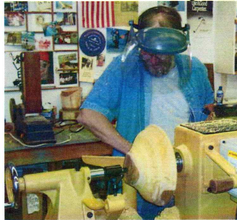
Ian takes a cut on the mulberry blank. In the background is the belt sander that Hank uses for sharpening gouges
