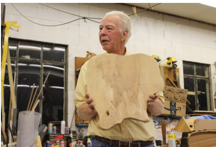
Bottom- Ken has a serving tray which he turned as a commission piece. He lightly turned each side to true up the surface but it subsequently warped. He then used 2 x 4's on each side in a vise and cranked the vise a little each day for over a week to get it flat. He spritzed both sides and will use Urethane Oil for a finish.
