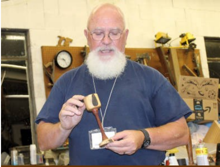
Charlie has a spalted maple cup with a spiral stem. He used a SORBY Micro Spiraling kit. Stem is mahogany.
