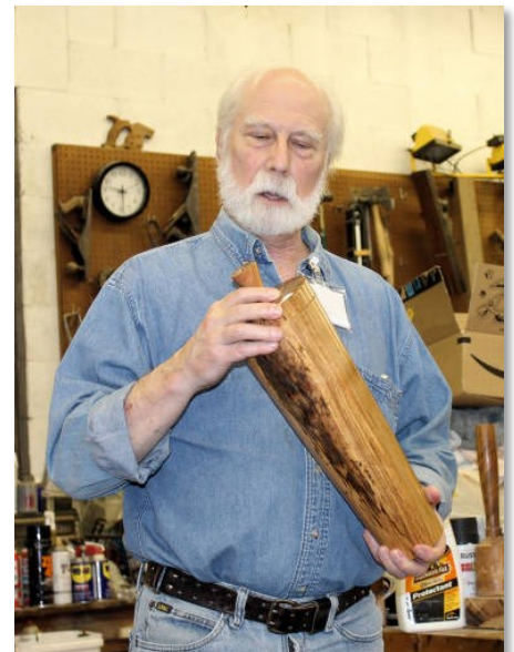
Andy holds a large hollowform turned from Hingham wood. He used a steady rest in the turning process. His turning tool was a hollowing rig by Steve Sinner. It has a urethane oil finish.
