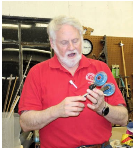
Wayne has a bracket made with skate wheels which you place in the tailstock to turn off the tenon with adapters. It is called a "Tailstock Steady" and sells for $150.
