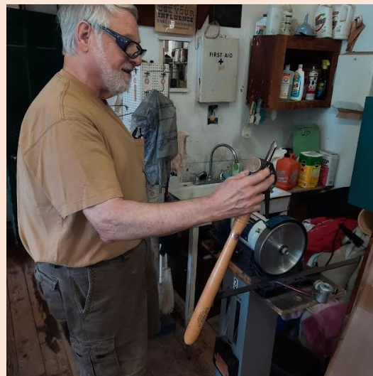
Wayne adjusts the jig holding his bowl gouge prior to sharpening it.
