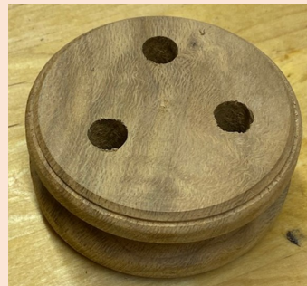
Prototype of a Deadeye (1 of 24) to be turned by MSSW in support of the Acorn to Arabella Project
