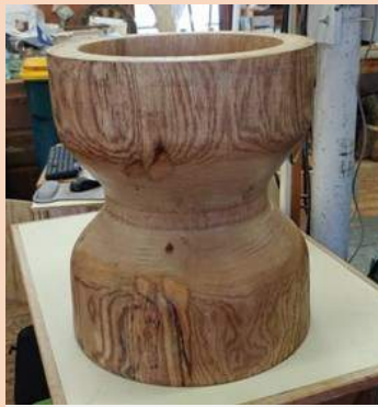
Air-dried over 1 year, the usu was ready for final turning.
