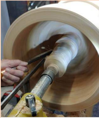
Tailstock supports the center spindle during hollowing.
