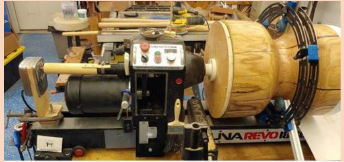
A rotisserie motor revolved the usu at 3 rpm to allow the epoxy to flow evenly over the interior surface.
