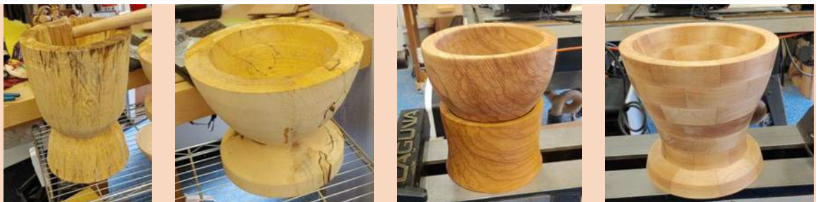
We considered several designs—including multipart and segmented. Ultimately we went with a single piece, hour-glass shaped design.
