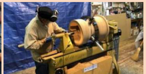
With the hourglass profile defined, we began the hollowing process.
