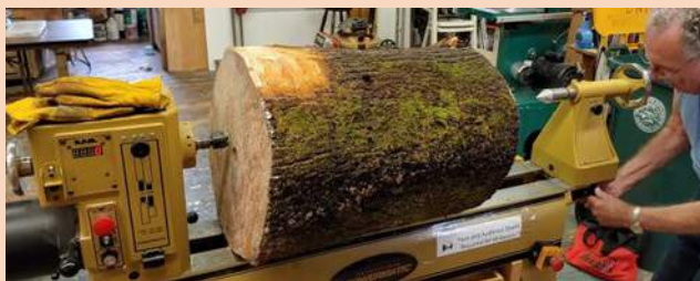
Steve Wiseman positioning the tail stock after the log is centered on the drive spur. We removed the bark for extra clearance and safety during turning.
