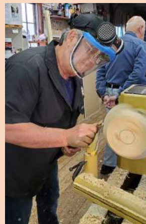
Joe demonstrates a shear cut
