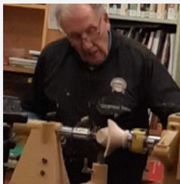
Shaping the dome.
