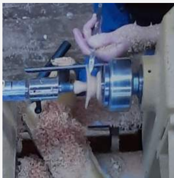
Steve shapes the under side of the tri corner into a convex surface before then finishing a concave cut on the tailstock side.
