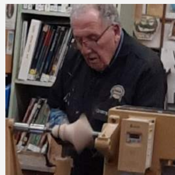
Steve is cutting a half round dome in preparation for drilling a half inch hole.
