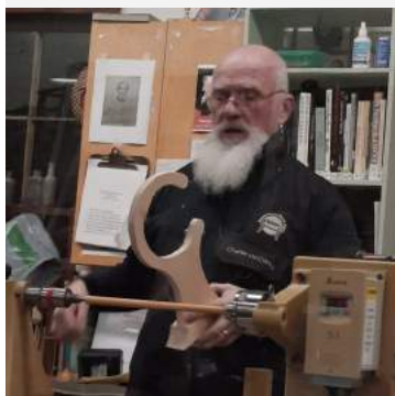
Charlie is holding a large steady rest to show us different features it has including magnets on the bottom. The "C" shape was made using a template
