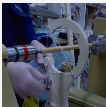
Charlie has his string steady rest all set up and ready to go. He can slide it to either side as he goes, which he said is necessary in being able to turn and finish only about an inch at a time.
