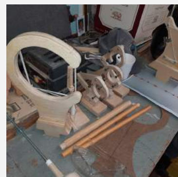
Charlie makes most of his steady rests. A few are shown here on the back bench.
