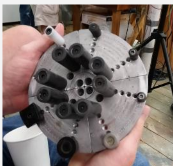
Closeup of the jumbo jaws expanded to illustrate the grabbing ability using the long padded stems inside as well as the smaller knobs outside.
