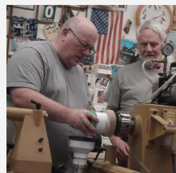
Wayne and Tim screw the vacuum chuck onto the lathe.
