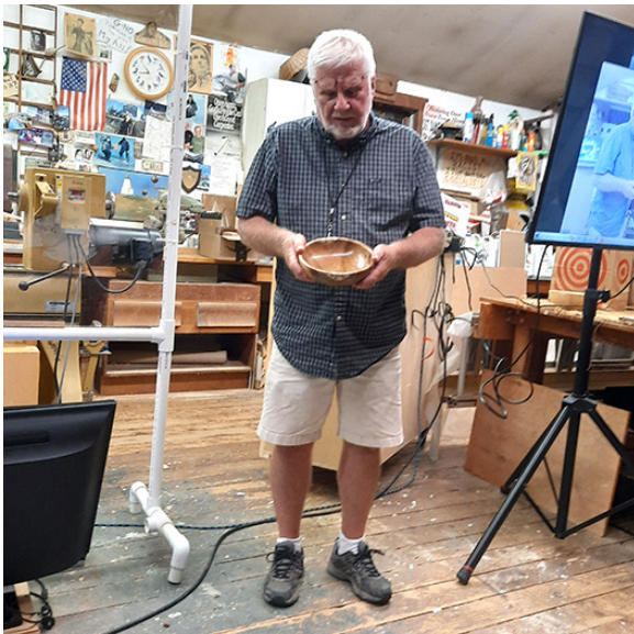
Sonny showed us this mahogany bowl he turned with maple branches inserted along the rim across from each other. Between the branches he used a soapstone inlay where the pith used to be. The soapstone came from Lee Valley. He glued them in using thin CA glue before giving it a final turn.
