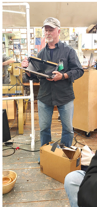
Carl also shared one of his attachments for dust control, using cardboard and acetate flaps to capture and direct shavings to the hood attached to his dust collector. Feel free to contact him for more details.
