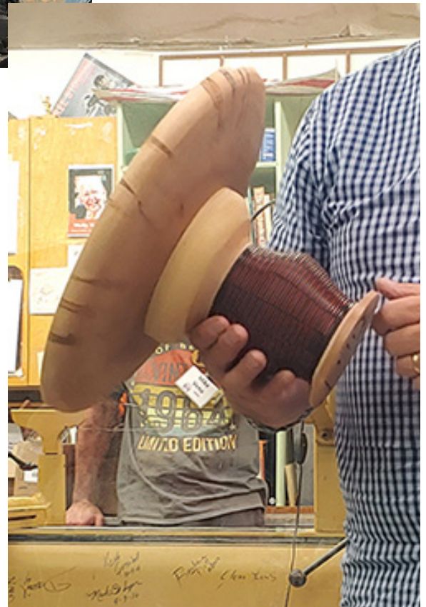
The second piece is a center-piece from a salvaged end-grain platter that puckered at the pith and a base embellished with a basket illusion created with a 3/16" beading tool, pyrography and india ink. All finished with wipe-on Polyurethane. The piece is a gift to a Special Education Class at Carver High School and the Rise & Shine inscription is their mission statement.
