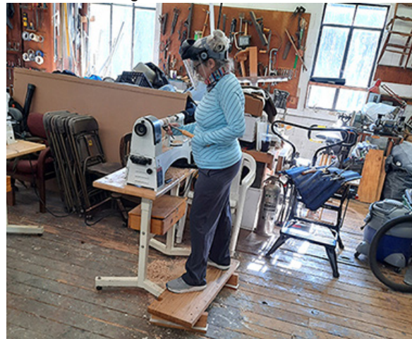
New member Angela van Laarhoven works on turning beads and coves on the lathe.
