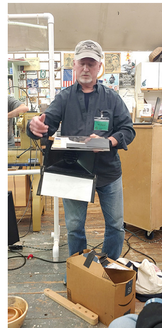
Carl also shared one of his attachments for dust control, using cardboard and acetate flaps to capture and direct shavings to the hood attached to his dust collector. Feel free to contact him for more details.
