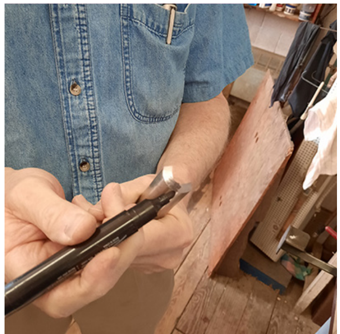
One of Wayne's techniques is to use a Sharpie to color the bevel of the gouge before applying it to the grinding wheel to make sure he gets an even edge.
