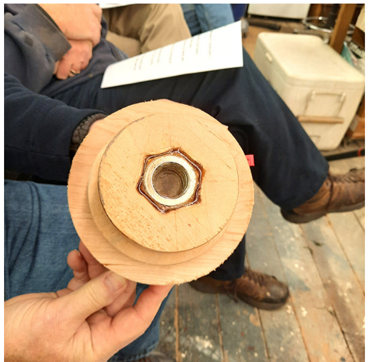
Pictured is the back of Steve's glueblock and blank using a nut embedded into the back to allow for screwing it onto the headstock.
