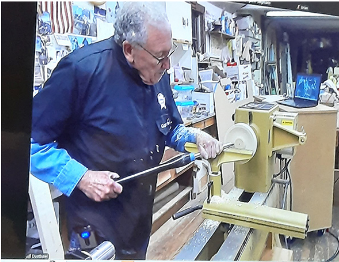
Steve hollows out around the tenon leaving a 3/8ths inch rim on the edge.
