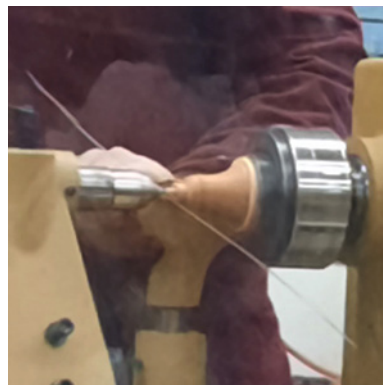
Here we see the bell in the jamb chuck and Bob is finishing the top.
