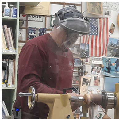
Bob turns a jamb chuck to hold the base of the bell so that he can finish the crown and shape the ball finial.
