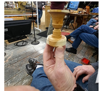
An inverted bell with tenon ready to have the top finished.
