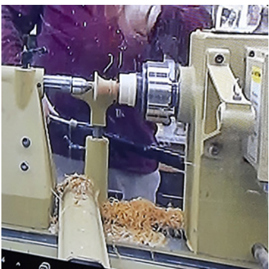
Bob uses a 7/8" Forstner bit to drill into the base of the bell.
