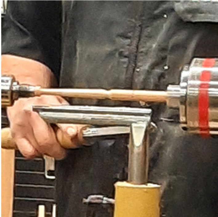
Charlie tapers the shaft of the pin, has formed the cove and rounded parts and is rounding the base near the point here.
