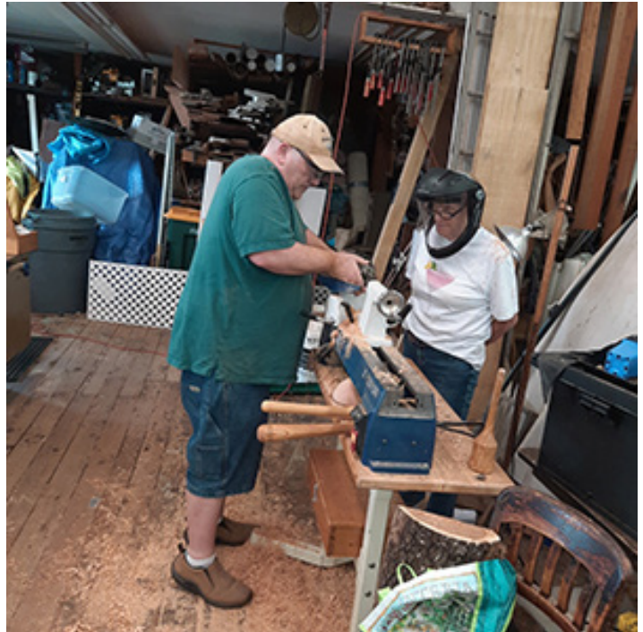
Tim Rix mentors a new member, Barbara, on installing a chuck on the lathe.
